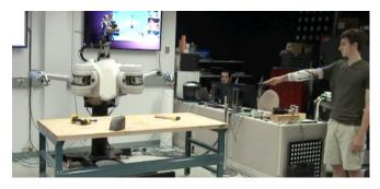
Fig. 4. Point-to-goal command to the manipulation robot: The user points to the impact driver of the left part of the table.
